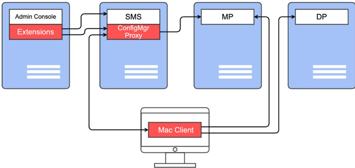
The arrow lines on the diagram represent communication channels between Parallels Device Management and Configuration Manager components.
