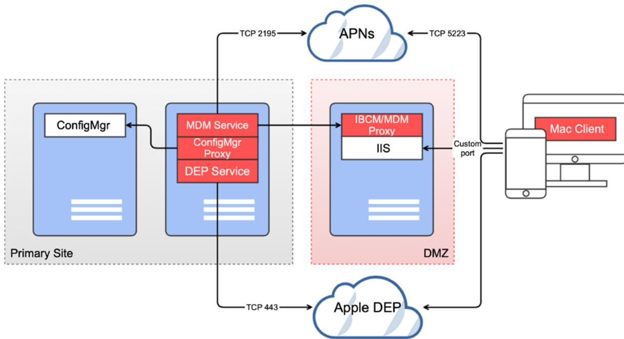
Please note that port numbers specified on the diagram are used for communications with Apple services and cannot be changed. Port numbers that are not specified (the Parallels IBCM/MDM Proxy ports) are configured when you run the Parallels IBCM/MDM Proxy Configuration Wizard.
